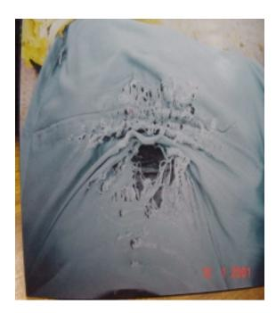
PHOTO 2 – "Búfalo" KEVLAR® SUIT AFTER TWO PASSES WITH UHP ROTARY GUN
