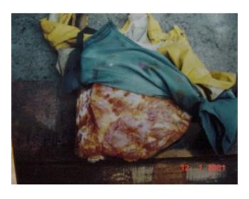
PHOTO 3 – AFTER TEST INTERIOR SIDE OF KEVLAR® SUIT. NO DAMAGE TO COW RIB WITH 40 MM (1.5 INCHES) OF FLESH
