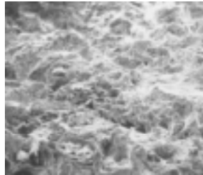
Figure: 6 Surface Shading from Inclusions of Dark Mineral Grit (Coal Slag)
