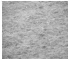
Figure: 6 Surface Shading from Inclusions of Dark Mineral Grit (Coal Slag)
